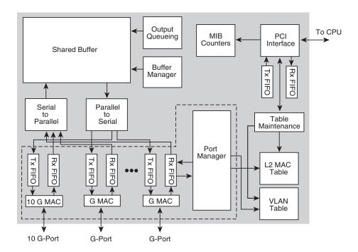
The BCM5632E switching processor chip supports 12 Gigabit ports and one 10-Gigabit uplink with all ports in wirespeed operation. The BCM5632E is ideal for applications such as multi-Gigabit port switches or aggregating multiple-Gigabit ports to a 10-Gigabit backplane.
